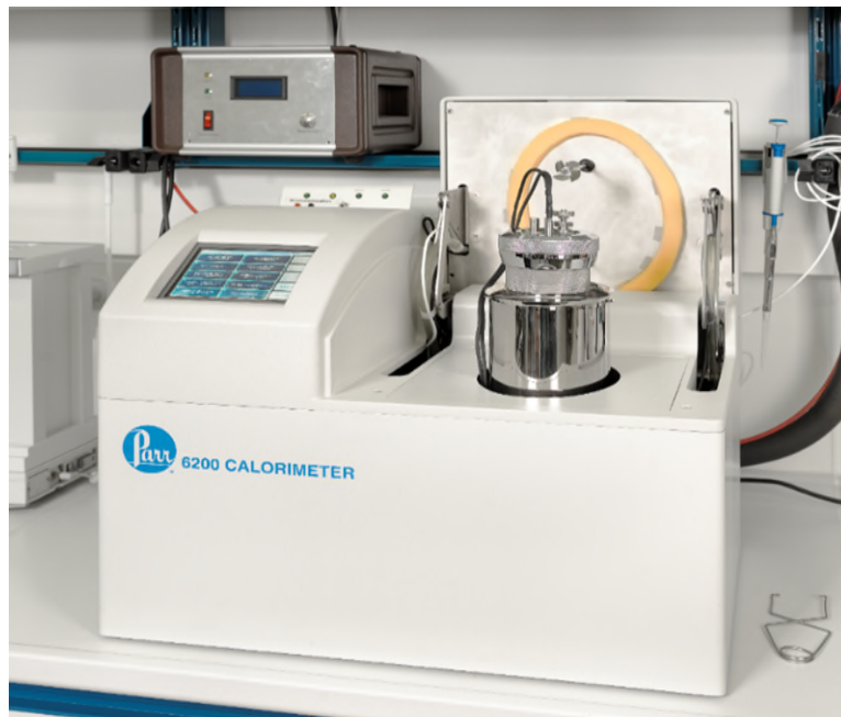
Figure 3. Example of an isoperibol calorimeter (Parr Instrument Company)
